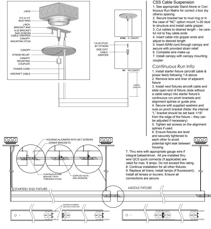
Note: To be installed by a qualified electrician per N.E.C. and all local codes.
