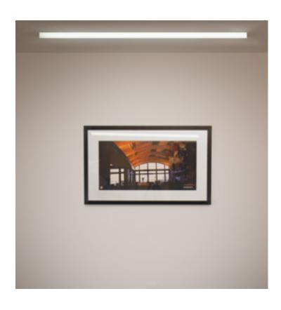
Elusive and revealing: JILL ASYM combines both qualities with a dropped-asymmetric lens designed to deliver wall-washing illumination from an ultraslender recessed aperture. JILL ASYM's 2-dimensional lens is designed to obscure lamp image on vertical side while simultaneously projecting wall washing light from the diagonal side of the frosted and clear prismatic acrylic lens combination.
